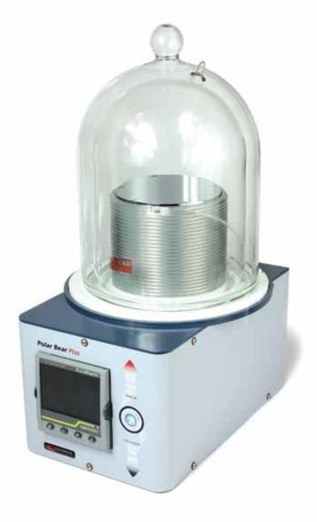
Developed in conjunction with the Innovative Technology Centre at Cambridge University, our Polar Bear *Plus* Flow Synthesiser has been designed to accurately deliver a range of hot and cold temperatures, for all your flow chemistry needs. The novel temperature control technology is clean and simple, requiring just a standard electricity supply for operation – no peripherals or consumables are necessary.
